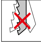
Switch off pendulum stroke
