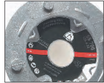
The steel CMT backing plate.
