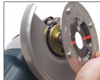
Place the backing plate on your angle grinder.
