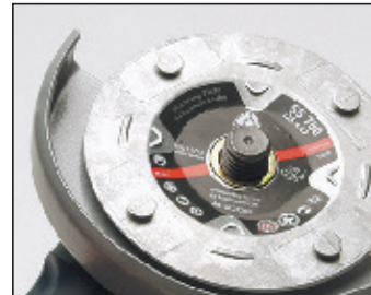
CMT backing plate on angle grinder.
