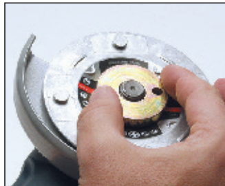
Use your standard locking nut to fasten the backing plate in place. (note: tighten locking nut with spanner wrench. Do not hand tighten)
