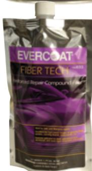
is a unique repair filler formulated with a combination of Kevlar and high tech short and long strand fibers. It offers superior strength and adhesion for repairing galvanized steel, aluminum, SMC, rigid plastic body panels, i.e., ground effects, spoilers, running boards, fenders, hoods, etc. FIBER TECH Reinforced Filler is waterproof, which makes it ideal filling weld areas, panel bond seams and rust damage.
