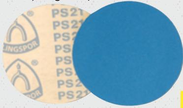
Extra long life and fast cutting for blending and shaping of body fillers, bare metal, welds and stripping paint. F-weight paper, fully resin-bonded, alumina zirconia grains. Ideal on steel and stainless steel plates. Also for use on stamped parts, final grinding of cast-iron housings.
