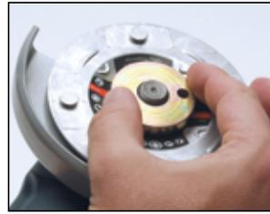
Use your standard locking nut to fasten the backing plate in place.
