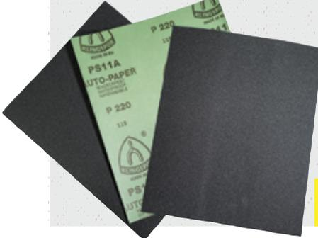
Sanding primer, clear coat, or plastic components. Waterproof Silicon Carbide, A and C-weight latex papers, resin-resin bonded and available in grits P60 - P2000. Use for sanding of furniture finishes such as varnish, lacquer, shellac, oil, polishing of glass, and in automotive body shops for final color sanding of paint.
