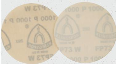
Perfect for excessive body filler sanding including paint, varnish, fillers and plastic. Heat Treated Aluminum Oxide on a 3 mil poly film backing, FP73W is the latest generation in the PS73W material product line. It's semi-open coat grain covering and double layer of stearate make it the ideal product for longer life in woodworking, solid surface, auto body and composite markets. The 3 mil poly film backing makes it tear resistant and enhances the finishing characteristics of this product.
